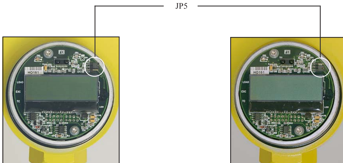
Figure G JP5 factory set for RS232 interface
